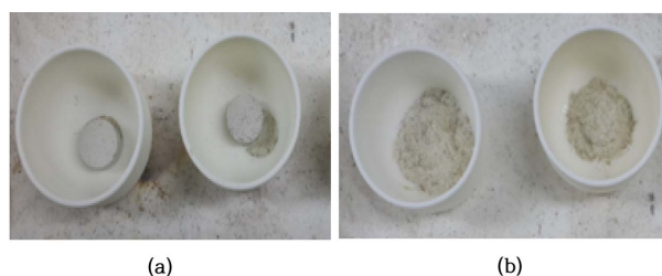
Fig. 2. Dusting responses during cooling after sintering: (a) Before Sintering, (b) After Sintering
